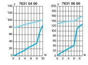
Direction of adjustment Return F: Flow in NI/min N: Number of turns
