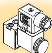
Valve is fitted with a 30mm solenoid having DIN 43650 Industrial form A. Operator body in thick anodised aluminium, stainless steel screws and armature allows compatibility with Railway applications.
