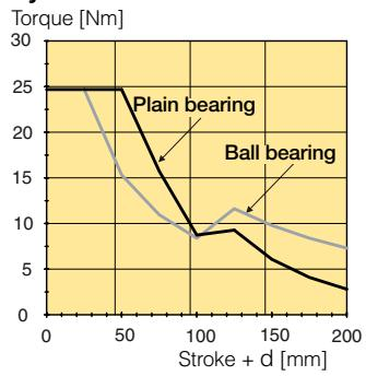
**Cylinder bore 80 mm**
