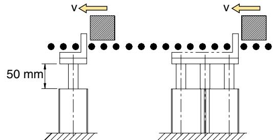
**Load stopping capacity as a function of speed**
