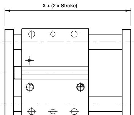
Please note that load capacity increases with two fixing plates, due to greater bearing distance.
