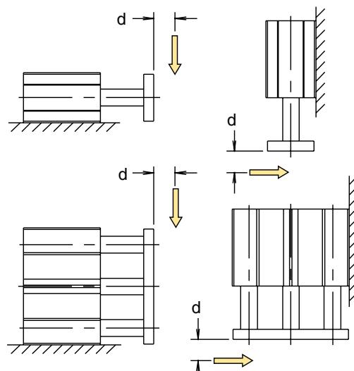
**Load capacity as a function of Stroke + d**
