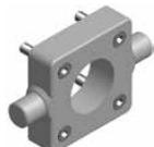
Intended for articulated mounting of cylinder. This trunnion can be flange mounted on the front or rear end cover of all P1D cylinders.
