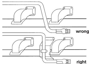
Avoid installing hose assemblies close to heat sources. However, if this should be required, insulate hose.
