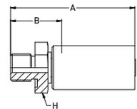
**MATERIAL** High strength carbon steel, zinc plated, C: Stainless steel
