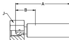
**MATERIAL** High strength carbon steel, zinc plated, C: Stainless steel
