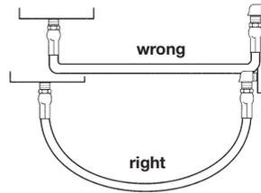
Hose should exit coupling in a straight position rather than side loaded. The minimum bend radius must not be exceeded to avoid kinking of hose and flow restriction.
