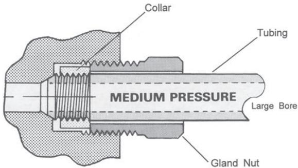
**Medium Pressure** is a 58/60° coned and threaded tubing design. *They have a maximum working pressure rating of 20,000 psi.*
