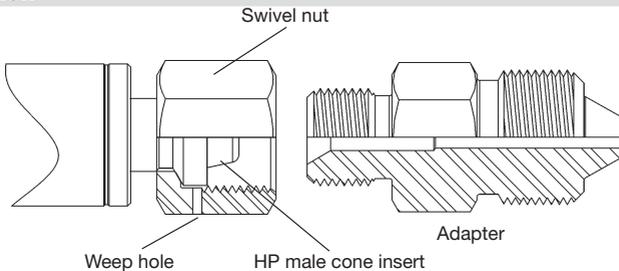
The Type “M” Swivel End Fitting is a swivel nut fitting with a 58° male cone nipple.
