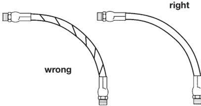
Hose is weakened when installed in twisted position. Also, pressure pulses in twisted hose tend to fatigue wire and loosen fitting connections. Design so that machine motion produces bending rather than torsion.
