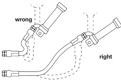
When hose assembly is installed in a flexing application, remember that metal hose fittings are not part of the flexible portion.
