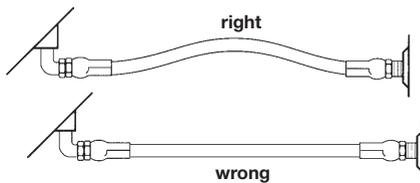
Pressure can change hose in length by as much as  $\pm 2\%$ . This must be considered when cutting hose to appropriate length.
