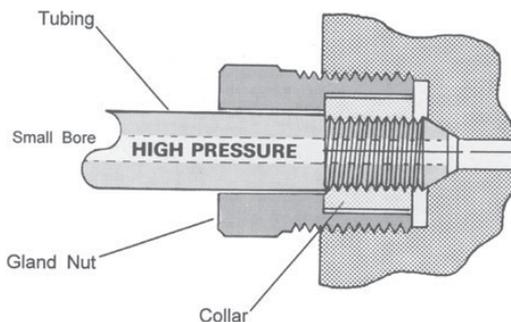
**High Pressure** is a 58/60 degree coned and threaded tubing design.
